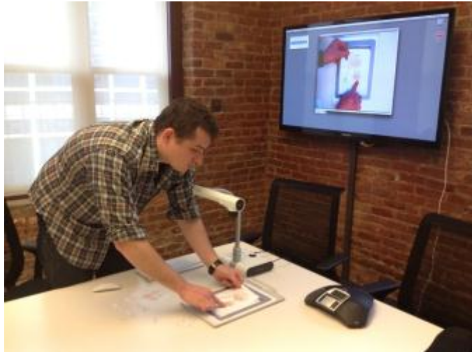
Fig. 2 Collaborating with the remote user using a document camera, a telepresence application capable of sharing images and audio, and a reconfigurable paper prototype.
