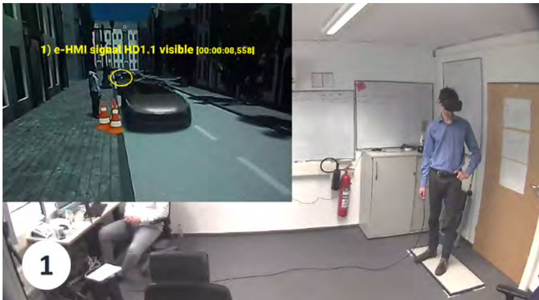
Figure 21. Example of measurements in VR – Visibility time of e-HMI signal HD1.1. (source: Rasmussen, Rothmüller & Vendelbo-Larsen, 2018)
